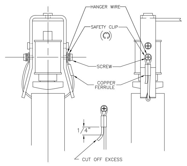
AFTER ADJUSTING CABLE FOR PROPER TUBE HEIGHT, BE SURE TO FORM CABLE LOOP LARGE ENOUGH TO SLIP OVER PHILLIPS HEAD SCREW, YET SMALL ENOUGH TO PREVENT IT FROM SLIPPING OVER THE SAFETY CLIP. CRIMP THE COPPER FERRULE WITH AN ADEQUATE SIZE TERMINAL CRIMPER. TRIM EXCESS CABLE AS SHOWN FOR NEAT APPEARANCE.
