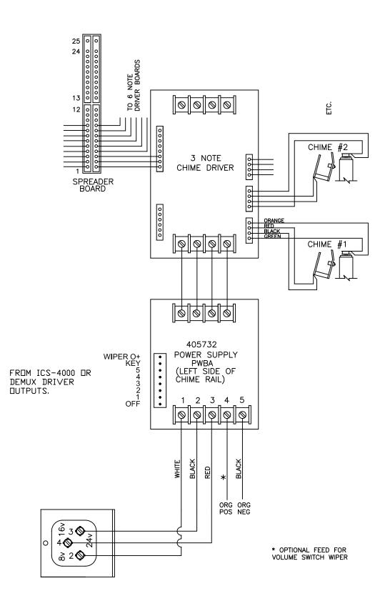
FIGURE 1 CHIME WIRING DIAGRAM
